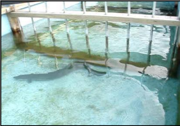
Figure 30: Eel being repelled by electric barrier in an experimental flume. (Photo: J. Boubée, NIWA)
