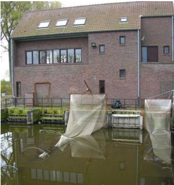
Figure 36: Fyke nets installed on the pump outlets to capture eels passed by the Archimedes screw pumps at the Buyse et al. 2014 study site. Note the pump set up appears to comprise five adjacent screw pumps (3 large/2 small) housed within the pump house pictured (photo – Google Earth).
