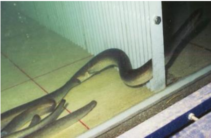
Figure 9: European eels (length 0.7 to 0.9m) passing through an intake screen grate with 20mm spacing and approach velocity of 0.9 to 1.0m/s (photo - U. Dumont)
