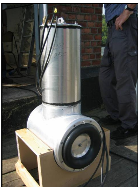
Figure 33: Infrasound module (ProFish 2 ). (photo – Profish)
