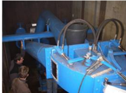
Figures 40 & 41: Venturi pump concept and actual pump produced by Fishflow Innovation. The main pump can be an existing one thus increasing the pumping capacity of the station. The intake to the pump needs to be protected by fine screens or other proven fish exclusion device. (from - http://fishflowinnovations.nl/en )
