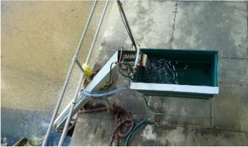
Figure 49. Fish trap and ramp, Waitaki Dam. Note that when operating the trap is covered with a shade cloth to keep the water cool and to keep predators at bay. (Photo N Blair, NIWA.)
