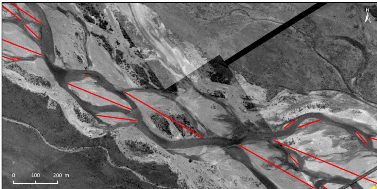
Figure 5: Lines drawn in ArcGIS Pro following the long axis of mid-channel bars in 1937. The total length of all lines in a reach was multiplied by two and then divided by the reach length to obtain a braiding index. The end of reach f can be seen at the bottom right of the image. Accurate assessment in some parts of the riverbed was difficult as a result of discontinuities (from the orthomosaic), lower resolution, and a lack of colour in the 1937 imagery, and over-exposure in some of the 2016-2018 imagery.
