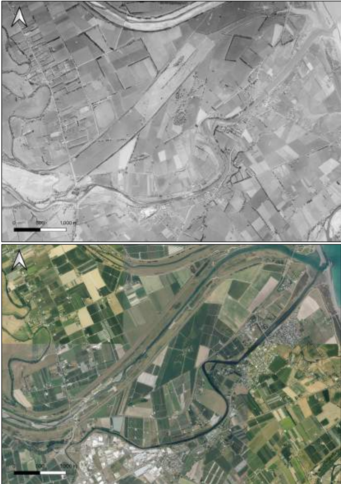
Figure 8: Ngaruroro and Karamū/Clive Rivers prior to diversion in 1937 (above), and following diversion in 2020 (below). Note where the main stem of the Ngaruroro used to flow past Clive and how it no longer has the capacity to do this, instead flowing through an extremely straight ‘flood channel’.
